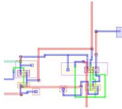
Figure 24: Layout Diagram of Comparator for tapped pin
