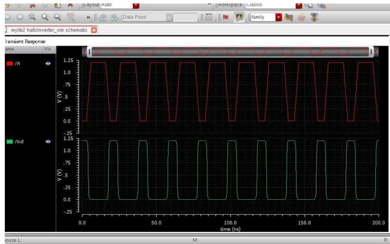
Figure 18: Simulation Waveform of Inverter
