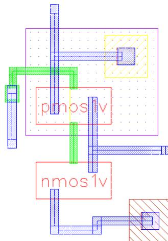
Figure 19: Layout Diagram of Inverter
