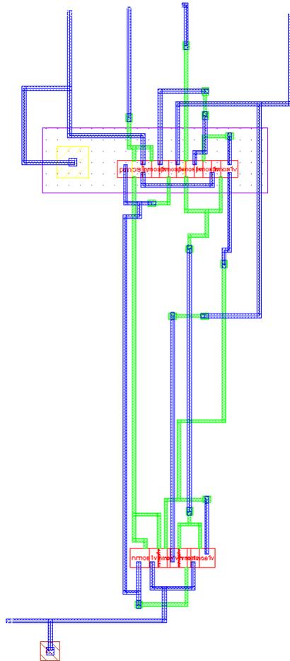
Figure 7: layout diagram of XNOR
