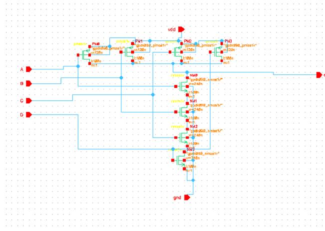
Figure 12: Schematic diagram of NAND
