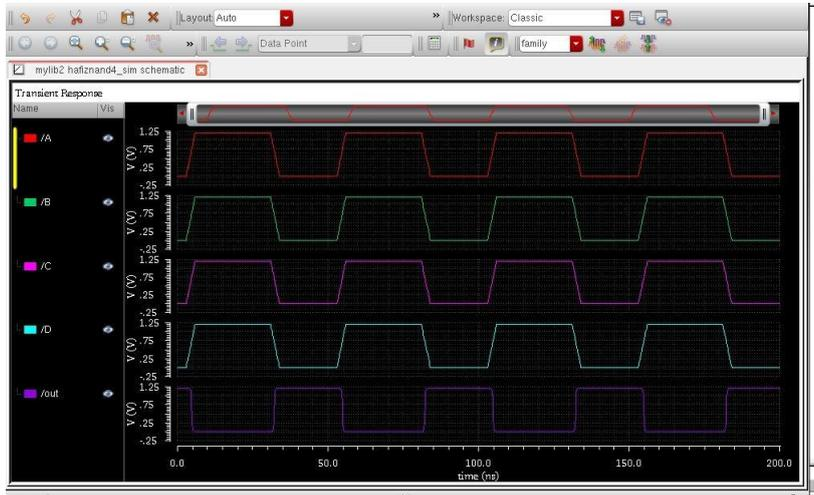
Figure 14: Output waveform of NAND
