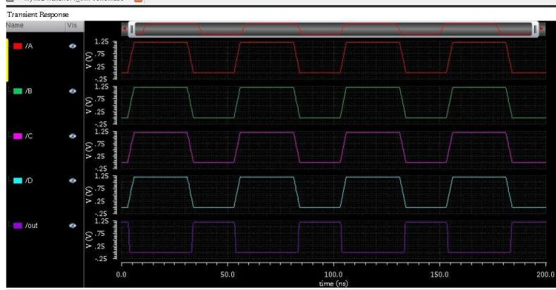
Figure 10: Output Waveform of NOR
