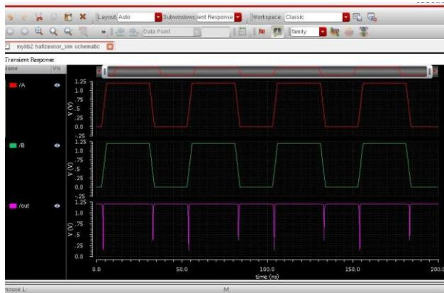
Figure 6: Output Waveform of 2-input XNOR
