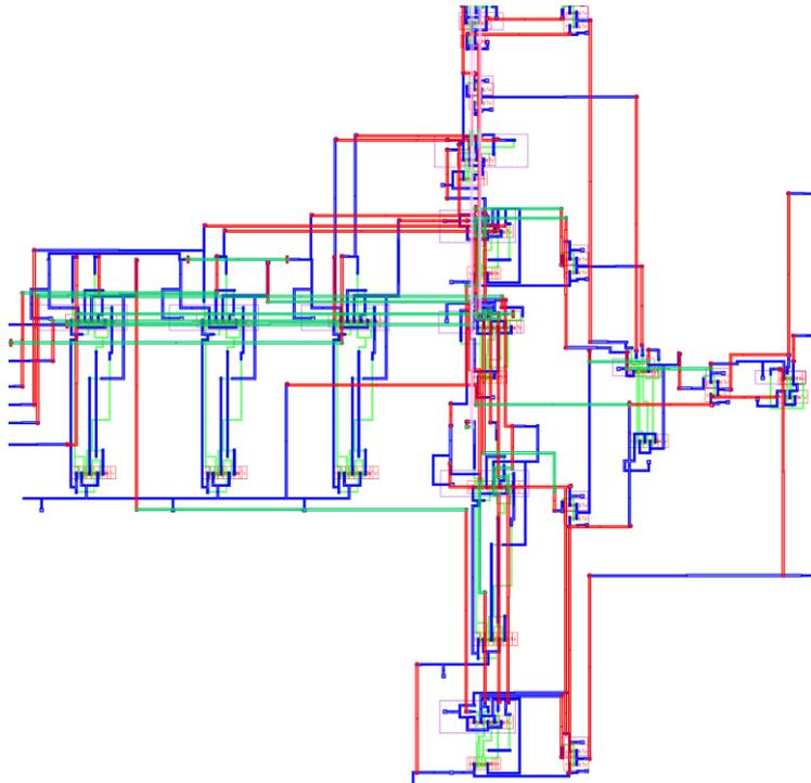
Figure 23: Layout Diagram of Comparator for Parasitic Capacitance
