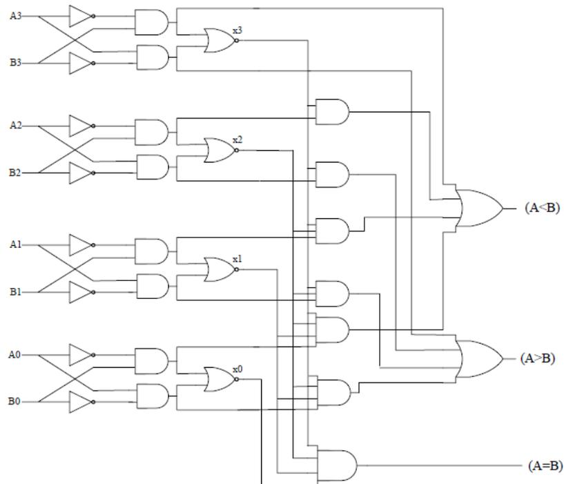
Figure 2: 4-bit Magnitude Comparator
