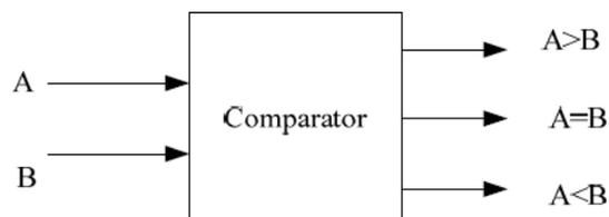
Figure 1: 1-bit Comparator
