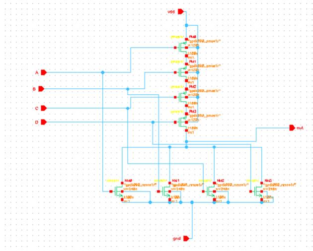
Figure 8: Schematic diagram of NOR
