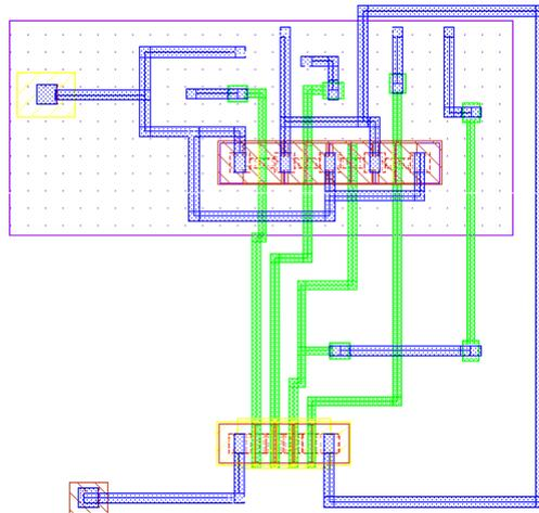
Figure 15: layout diagram of NAND
