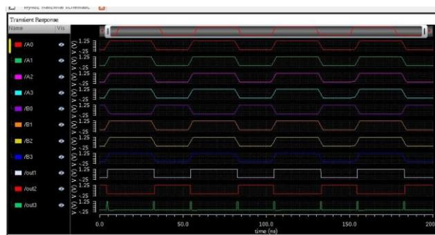
Figure 21: Simulation Waveform of Comparator
