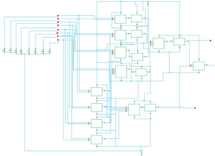
Figure 20: Total Schematic Design of Comparator
