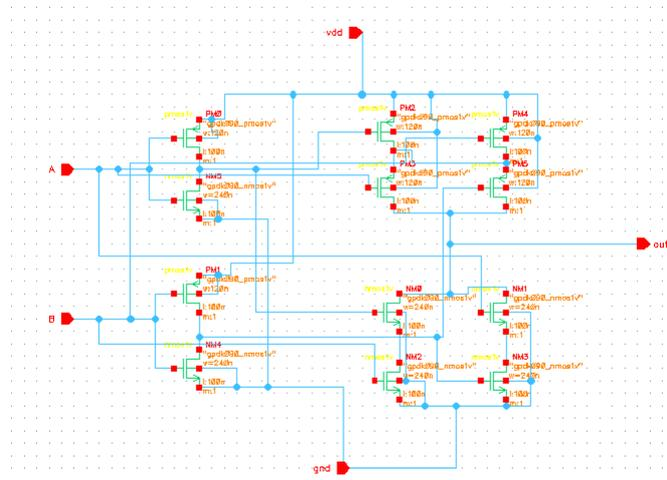
Figure 4: Schematic Diagram of 2-input XNOR
