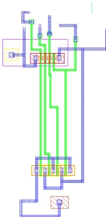
Figure 11: layout diagram of NOR
