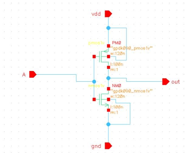
Figure 16: Schematic Diagram of Inverter
